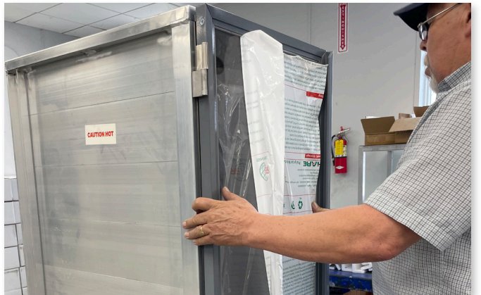
STEP 6 INSTALL DOOR TO THE CABINET (LINE UP HINGES' PIN HOLE)
