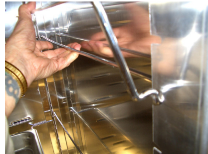
TILT THE RUNNER UP SLOWLY WHILE PULLING THE RUNNER OUTWARD AWAY FROM THE SIDE OF THE CABINET.
