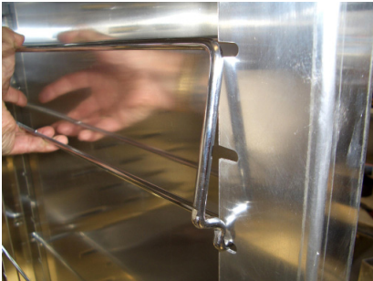
TILT THE RUNNER UP AND ENGAGE BOTH ENDS TOGETHER. DO NOT HAVE ONE SIDE ENGAGED LESS THAN THE OTHER.
