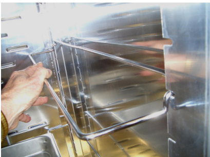
WHEN IN THE CORRECT POSITION THE RUNNER SHOULD BE AT 90 DEGREES TO THE SIDE OF THE CABINET.
